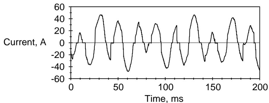
Figure 5.15 Input current waveform for the three phase cycloconverter operating at full motor load with 26 Hz output frequency.
