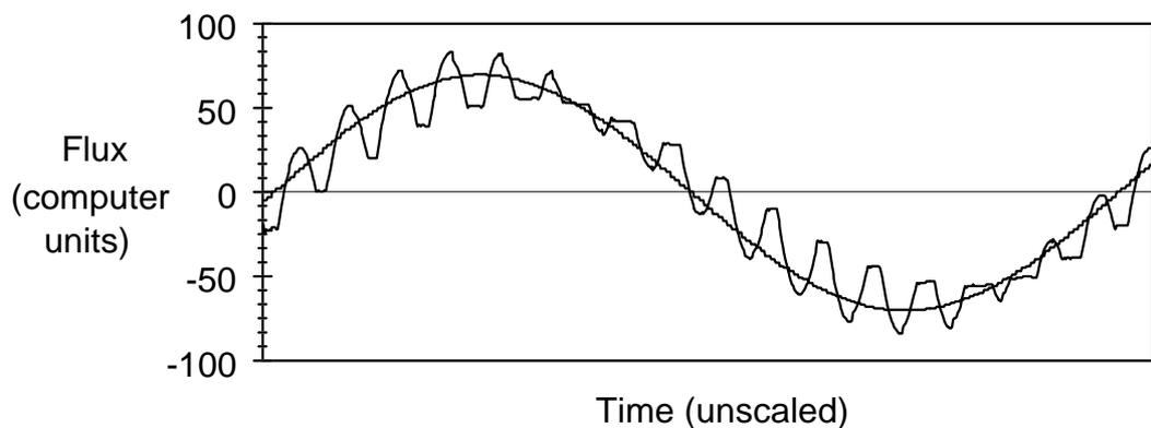
Figure 4.24 Computer derived output and reference flux waveforms for operation at 6 Hz and 0.9 Nm load.
