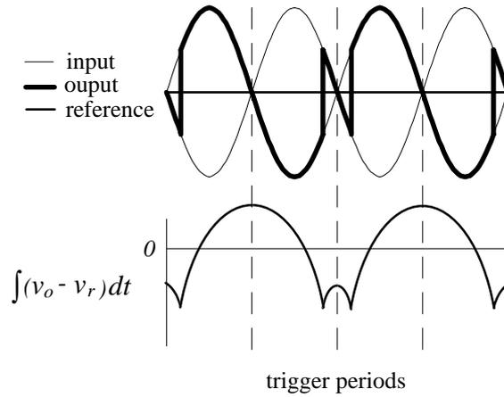
Figure 3.4 An example of instability in a 2-pulse cycloconverter that can occur for double integral control with no stabilising terms.
