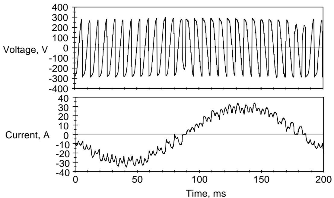
Figure 5.9 Output waveforms for the three phase cycloconverter operating at 5 Hz with a full motor load.
