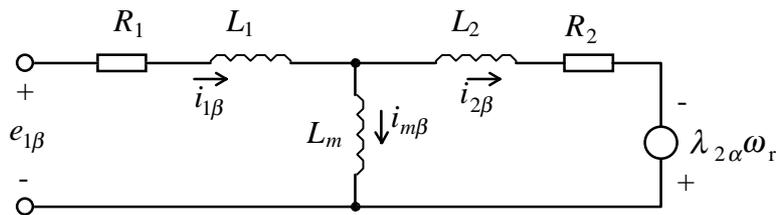
Figure 2.4 Equivalent circuit of the  $\beta$  phase.
