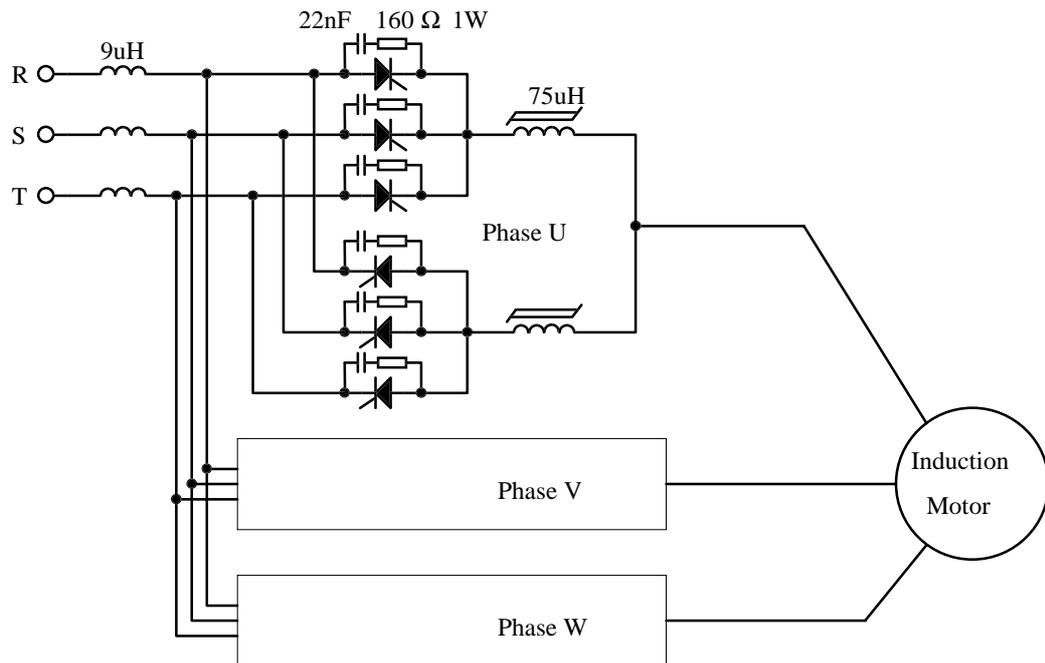
Figure 5.1 Power circuit of the 3-pulse cycloconverter
