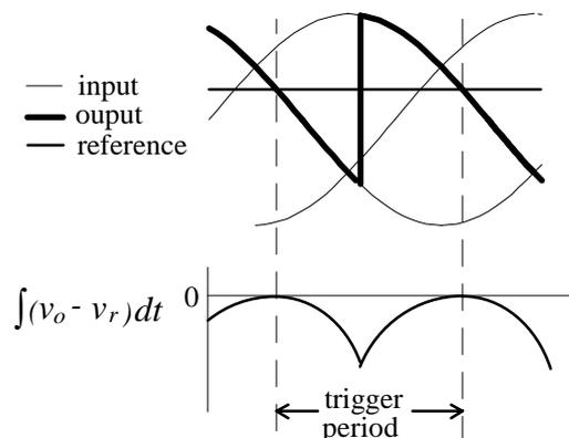
Figure 1.13. Illustration of the pre-integral control method for positive load current.
