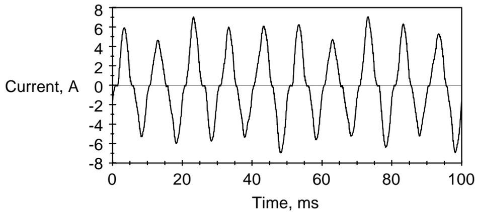
Figure 4.22 Input current waveform for the 1 to 2 phase cycloconverter operating at 20 Hz with a motor load of 1.4 Nm.
