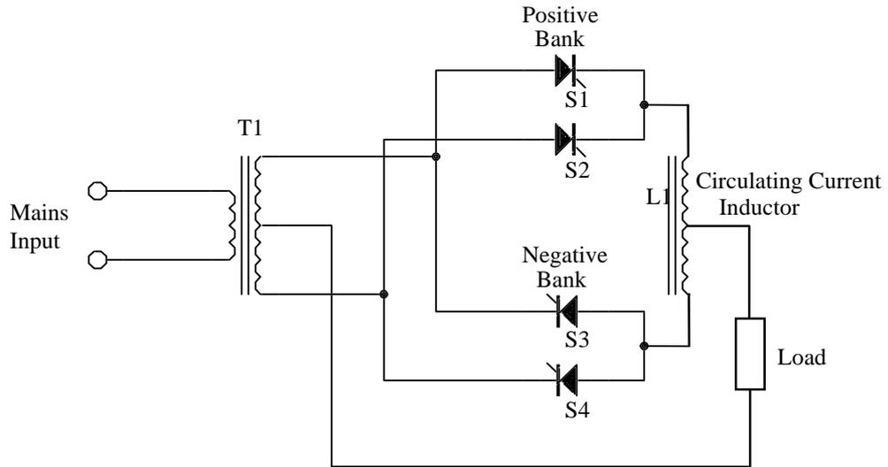
Figure 1.3 Two-pulse cycloconverter with circulating current inductor.
