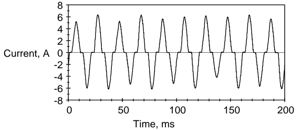
Figure 4.20 Input current waveform for the 1 to 2 phase cycloconverter operating at 6 Hz with a motor load of 0.9 Nm.
