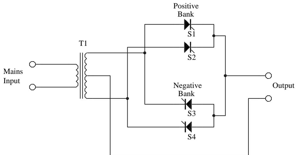
Figure 1.1 Basic single phase cycloconverter.
