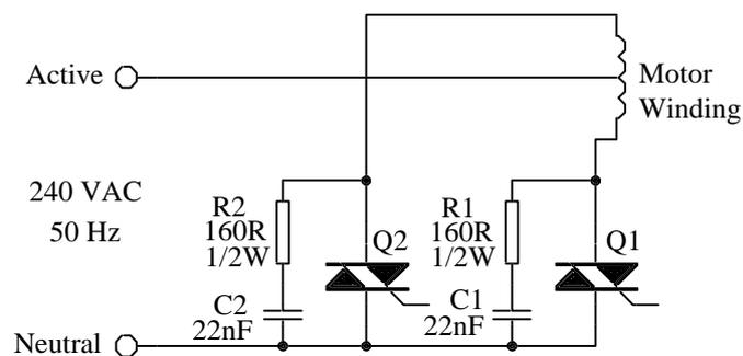
Figure 4.1 Complete power circuit for one phase of the cycloconverter
