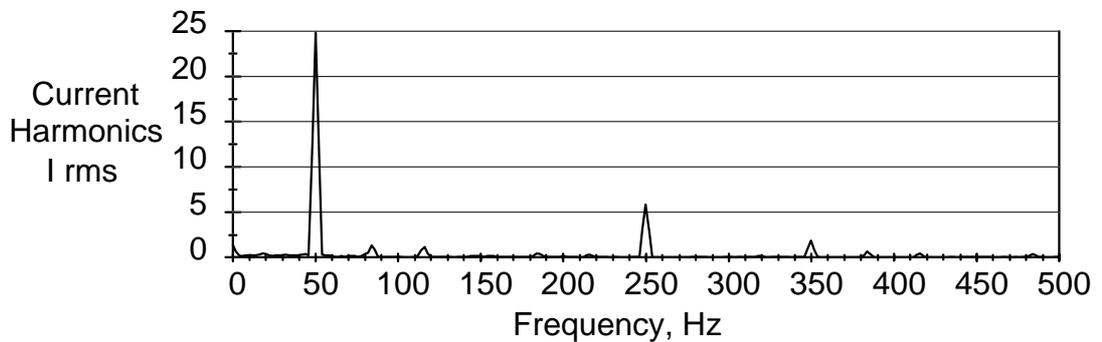
Figure 5.12 Frequency spectrum of the input current at full load with 5 Hz output frequency.
