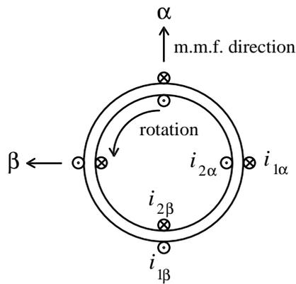
Figure 2.1 Basic two phase induction motor.
