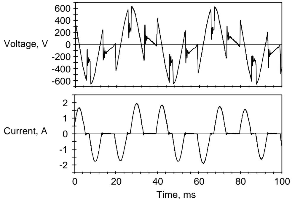
Figure 4.13 Output voltage and current waveforms for one motor phase of the 2 phase cycloconverter at 25 Hz with no load.
