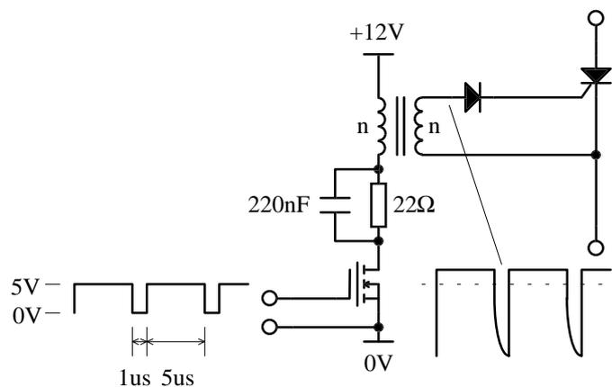
Figure 5.3 Gate drive circuit and waveforms.
