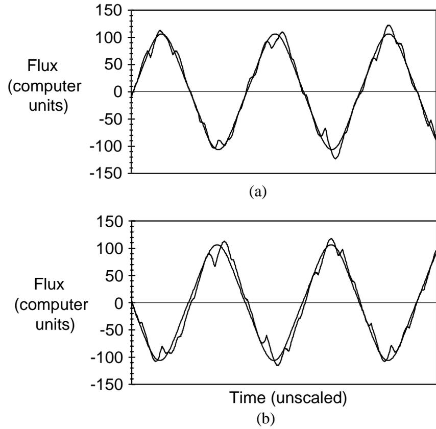
Figure 5.18 Feedback and reference flux waveforms at 20 Hz at (a) no load, (b) full load.
