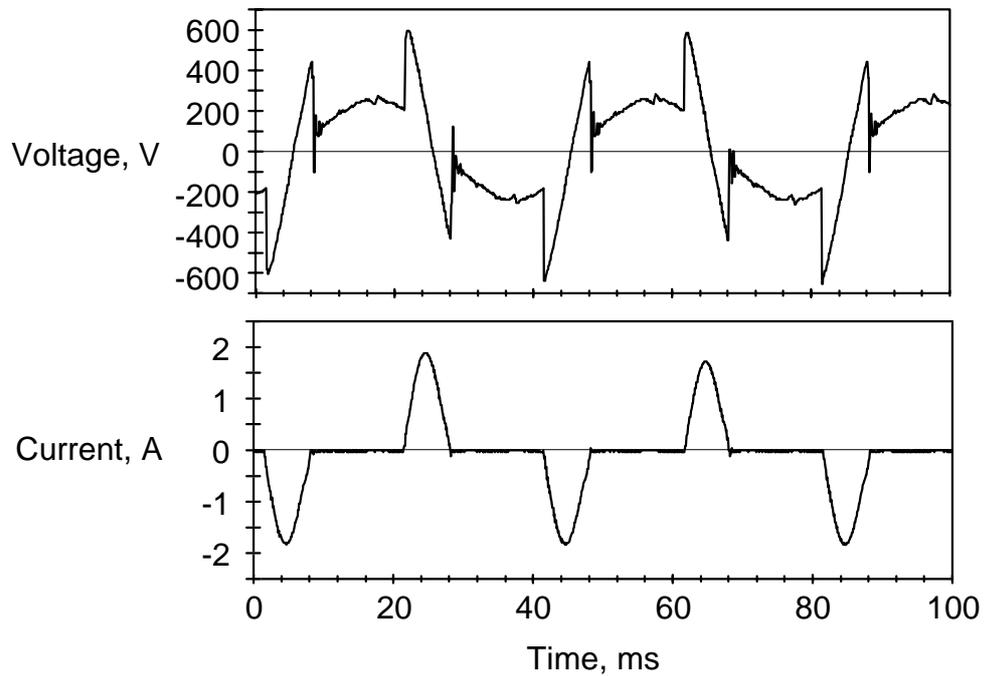
Figure 4.14 Output voltage and current waveforms at 25 Hz with a different input to output phase relation to Figure 4.13.
