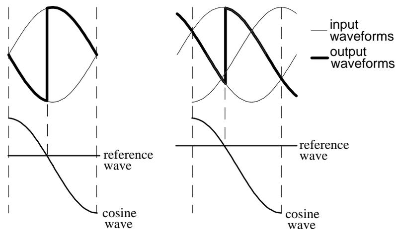
(a) Two-pulse cycloconverter (b) Three pulse-cycloconverter
