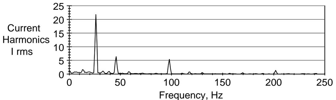
Figure 5.14 Frequency spectrum of the output current at full load with 26 Hz output frequency.
