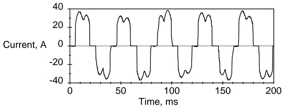
Figure 5.11 Input current waveform for the three phase cycloconverter operating at full motor load with 5 Hz output frequency.
