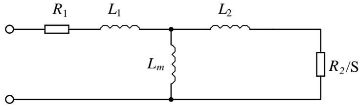
Figure 2.11 Classical steady state per phase equivalent circuit.
