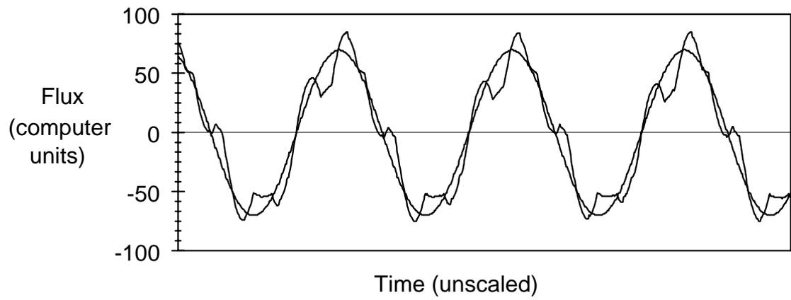
Figure 4.25 Computer derived output and reference flux waveforms for operation at 20 Hz and 1.4 Nm load.
