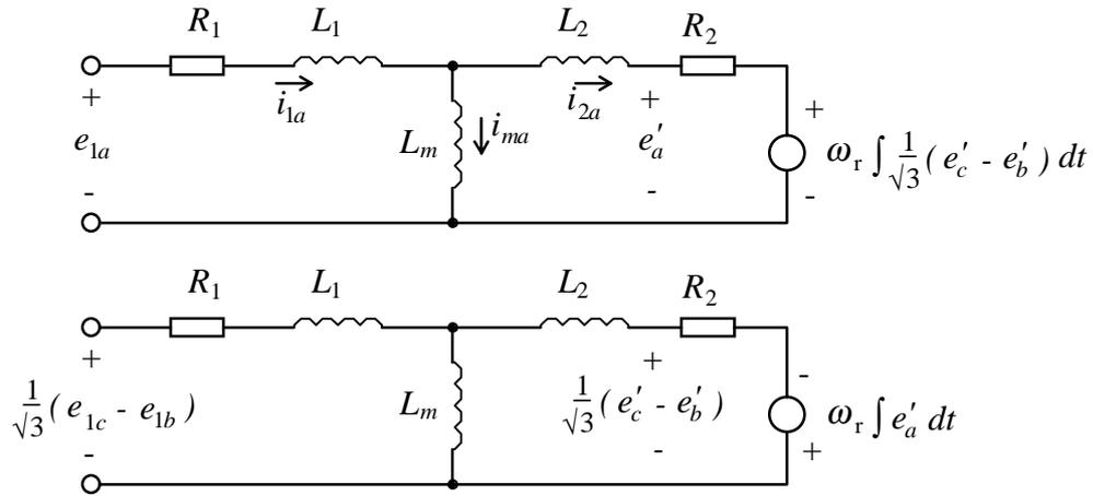
Figure 2.8 Two phase equivalent circuit with transformed variables. The  $\alpha$  axis is aligned with the  $a$  phase.
