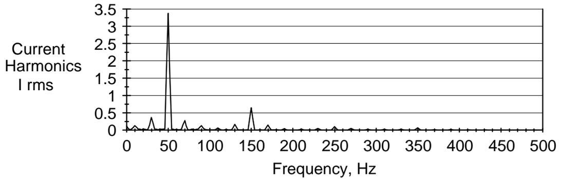
Figure 4.23 Frequency spectrum of the input current with 20 Hz output frequency.
