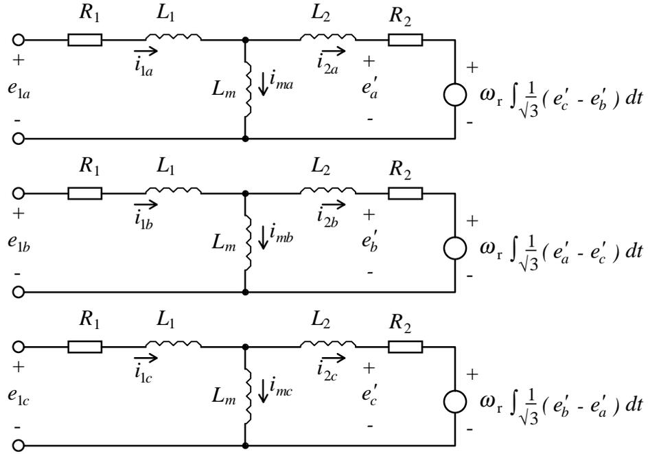
Figure 2.10 Three phase equivalent circuit.
