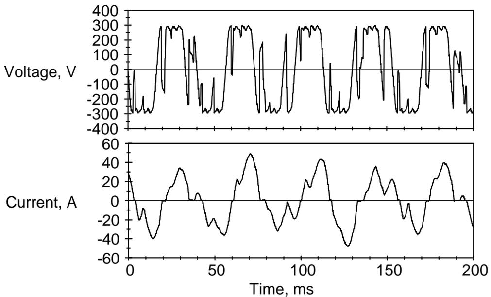
Figure 5.13 Output waveforms for the three phase cycloconverter operating at 26 Hz with a full motor load.
