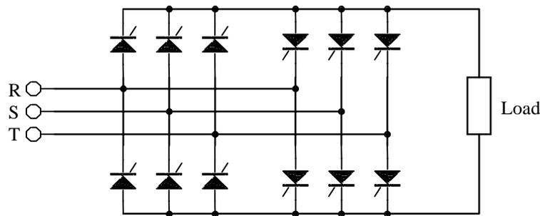
Figure 1.6 Three phase input, 6-pulse cycloconverter.
