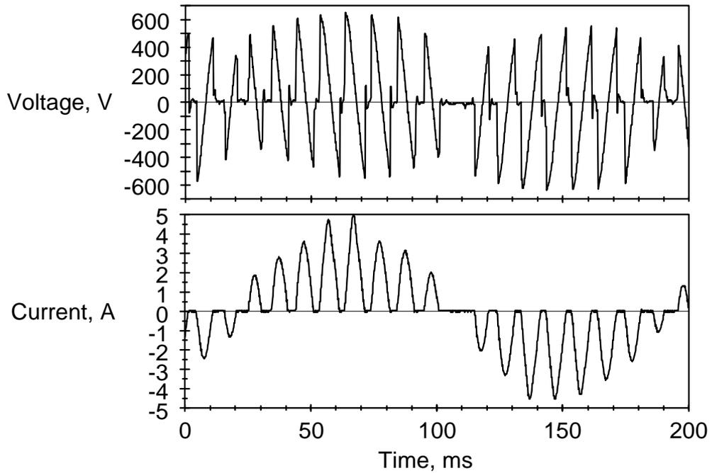
Figure 4.16 Output waveforms for one phase of the 1 to 2 phase cycloconverter operating at 6 Hz with a motor load of 0.9 Nm.
