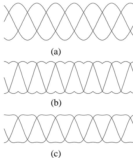
Figure 5.5 Possible waveforms for the output reference. Waveform (a) limits the peak line to line voltage, while waveform (b) has excessive  $dv/dt$ . The waveform chosen is (c).
