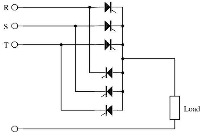
Figure 1.4 Three phase, 3-pulse cycloconverter.
