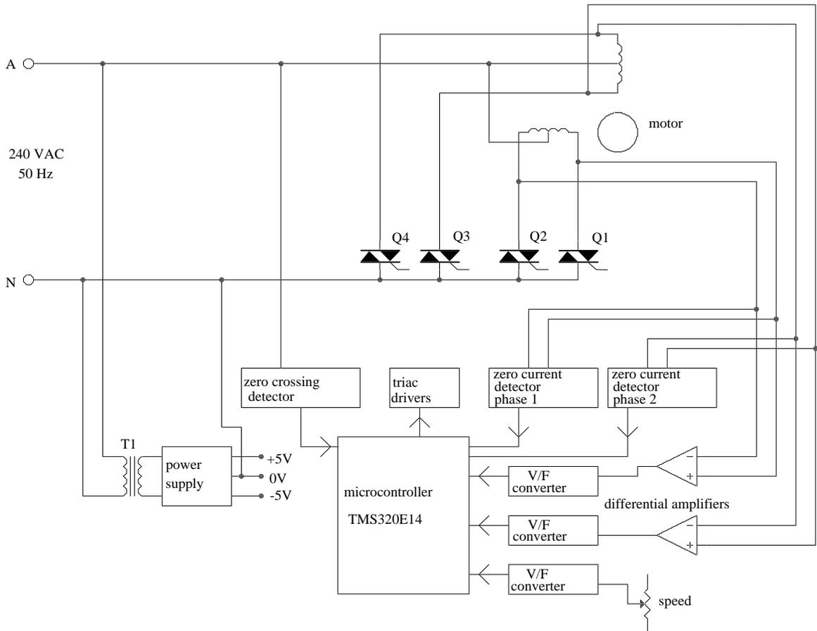
Figure 4.2 Block diagram of the control circuit together with a simplified power circuit.
