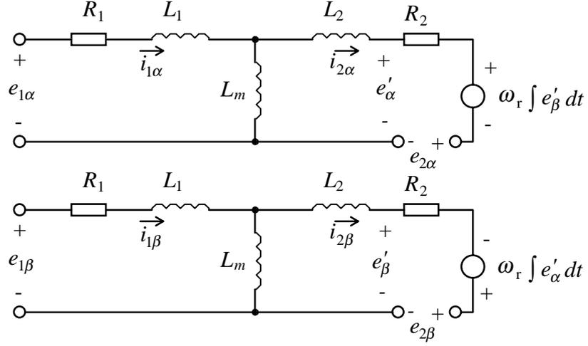
Figure 2.6 Equivalent circuit of the two phase induction motor with rotor voltages added for derivation of Kron's Equations.
