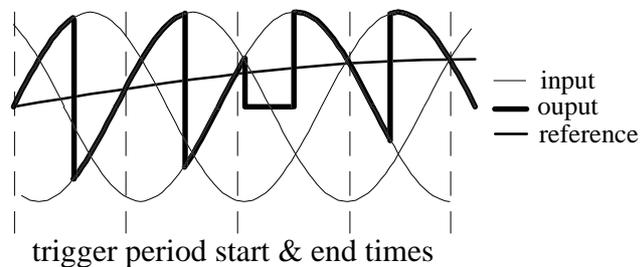
Figure 3.9 An example of bank cross-over from the negative to the positive bank for a 3-pulse cycloconverter showing the extended time between the start and end of trigger periods.
