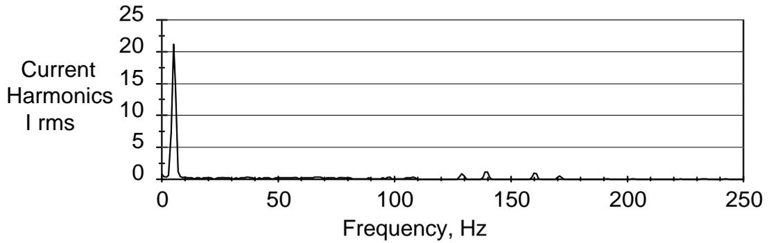
Figure 5.10 Frequency spectrum of the output current at full load with 5 Hz output frequency.
