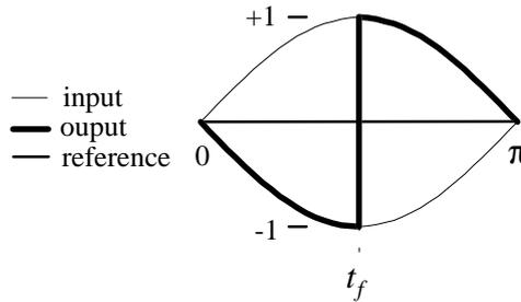
Figure 3.5 Normalised trigger period for the simulation used to determine the constant  $K$  for a 2-pulse cycloconverter.
