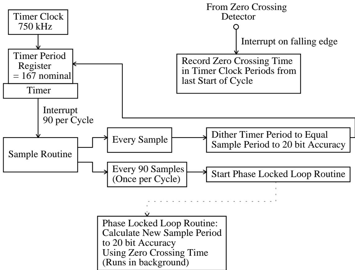
Figure 4.4 Block diagram of the phase locked loop operation.
