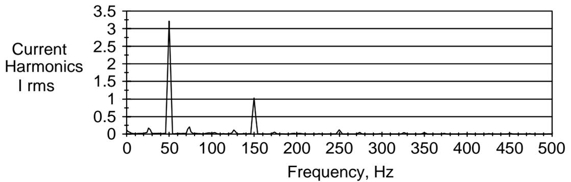
Figure 4.21 Frequency spectrum of the input current with 6 Hz output frequency.
