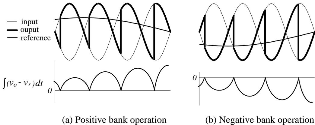
Figure 1.11 Waveforms obtained from a 2-pulse cycloconverter with integral control.
