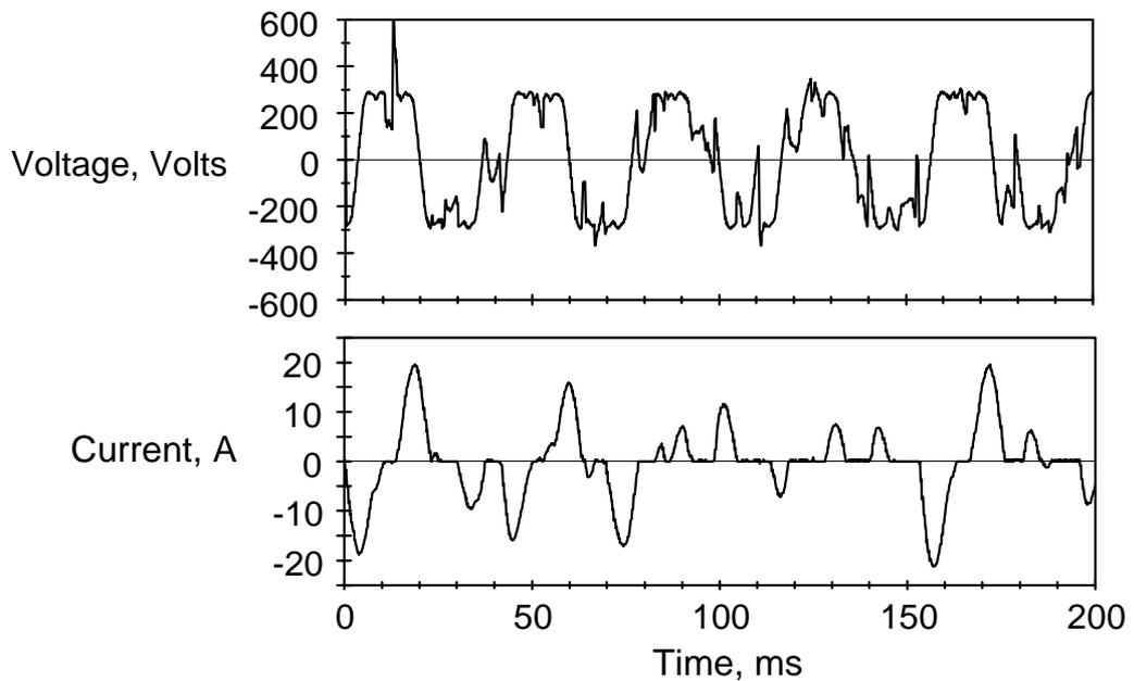
Figure 5.8 Output waveforms for the three phase cycloconverter operating at 26 Hz with no load.
