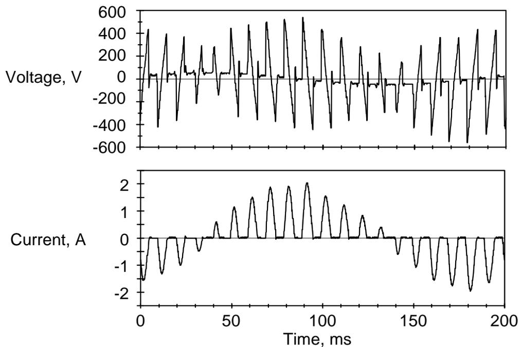
Figure 4.11 Output voltage and current waveforms for one motor phase of the 2 phase cycloconverter at 5 Hz with no load. The voltage is measured across both windings on the phase (and is thus twice the nominal phase voltage) and the current is the sum of the currents in both windings.
