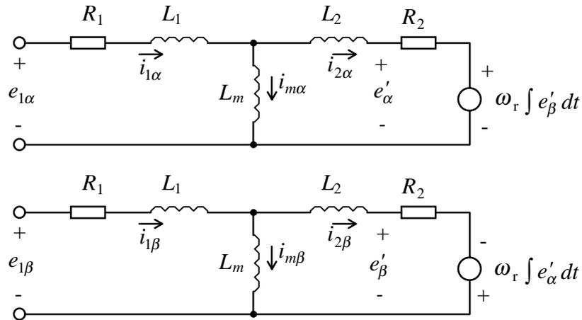
Figure 2.5 Final equivalent circuit of the two phase induction motor.
