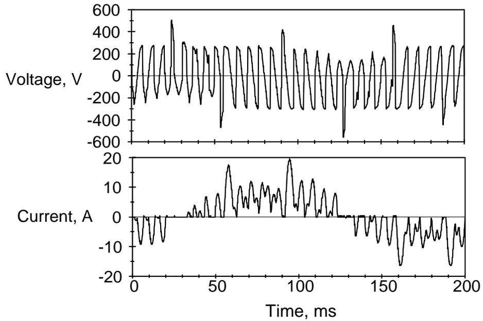
Figure 5.7 Output waveforms for the three phase cycloconverter operating at 5 Hz with no load.
