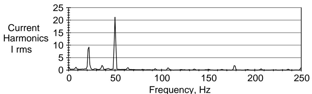
Figure 5.16 Frequency spectrum of the input current at full load with 26 Hz output frequency.
