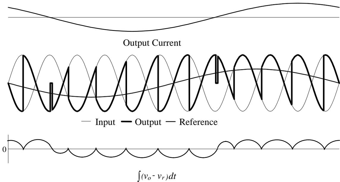
Figure 3.2 Illustration of distortion introduced with integral control
