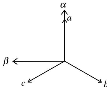
Figure 2.7 The superimposed three phase and two phase axes for the basic two pole motor.
