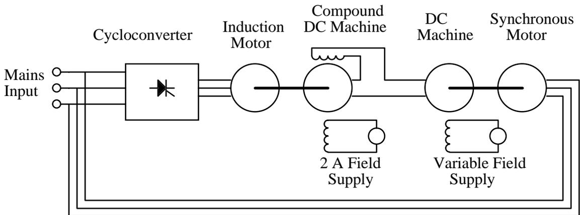
Figure 5.6 Equipment set-up for testing the 3 phase cycloconverter
