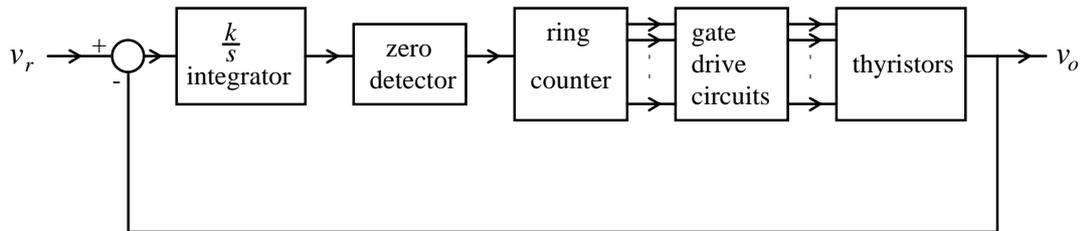
Figure 1.10 Block diagram of integral control.
