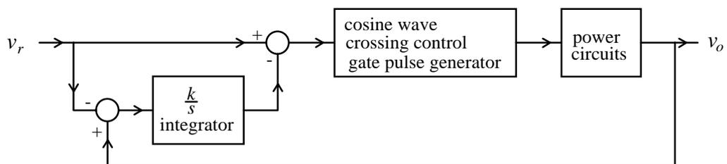
Figure 1.8 Simplified block diagram of ripple voltage integral feedback control scheme.
