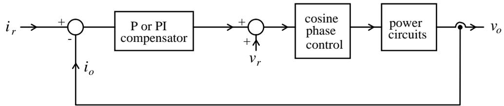
Figure 1.9 Simplified block diagram of current feedback control scheme.
