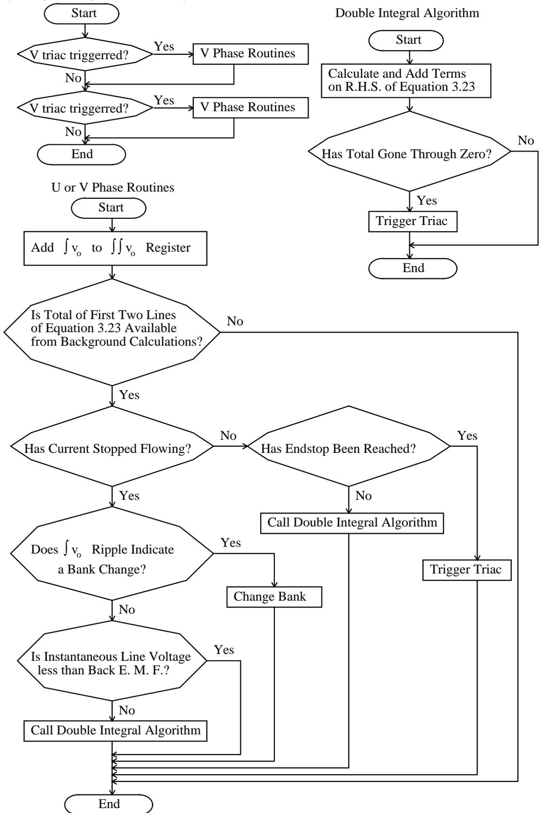
Figure 4.6 Tasks carried out at every sample except at the start of a half cycle.
