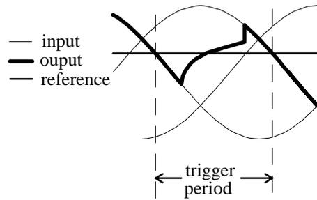
Figure 1.14 Pre-integral control with discontinuous current.
