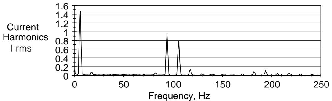
Figure 4.17 Frequency spectrum of the output current with 6 Hz output frequency.
