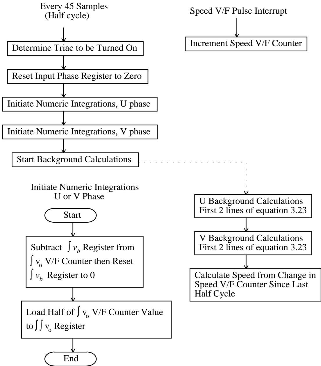
Figure 4.5 Block diagram of tasks carried out every half cycle sample and the related speed V/F software counter.
