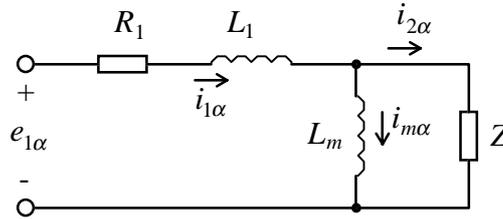
Figure 2.2 Partial equivalent circuit of the  $\alpha$  phase.
