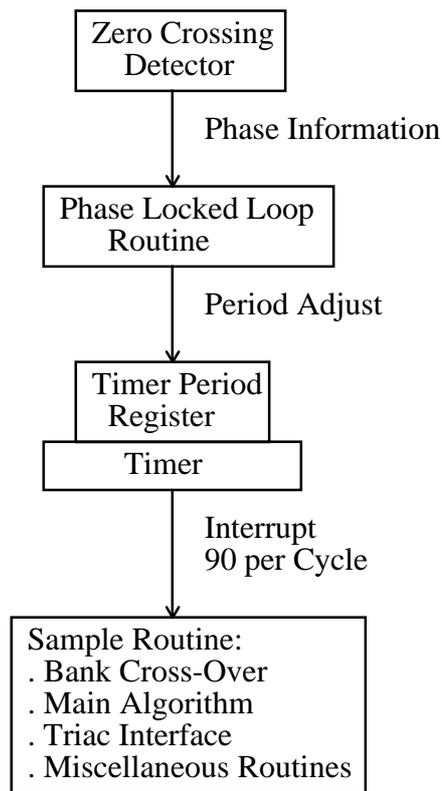
Figure 4.3 Block diagram of the software.
