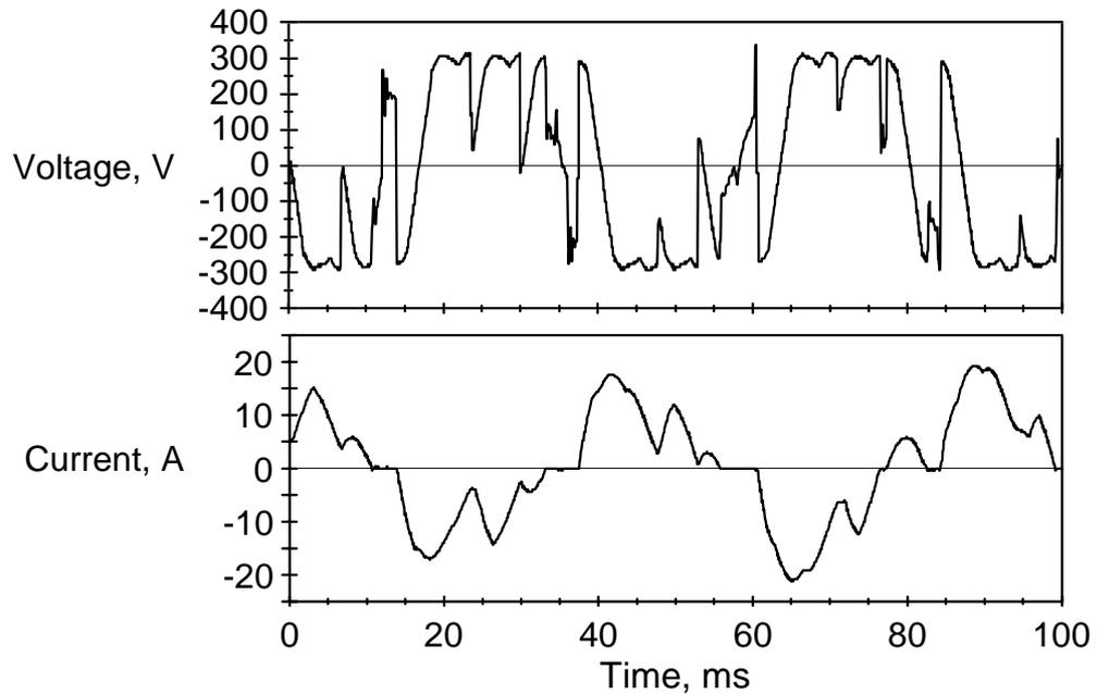
Figure 5.17 Output waveforms for the three phase cycloconverter operating at 22 Hz with a regenerative load.
